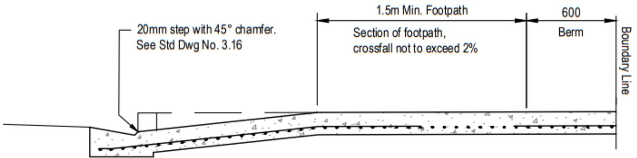
Concrete ramp reinforced with HRC 665 mesh,
