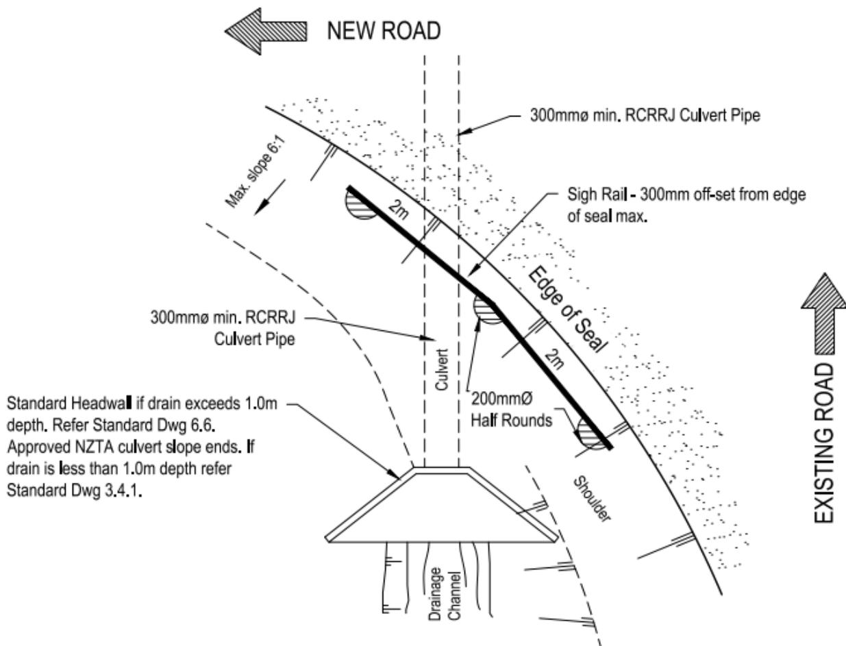
Standard Headwall if drain exceeds 1.0m depth. Refer Standard Dwg 6.6.
