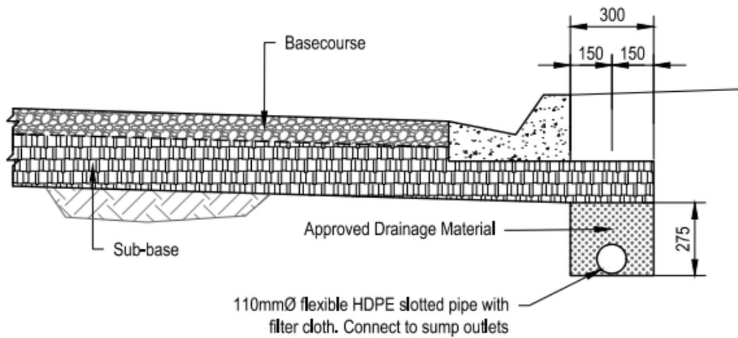
**SUBGRADE DRAINAGE DETAIL AT KERB**
