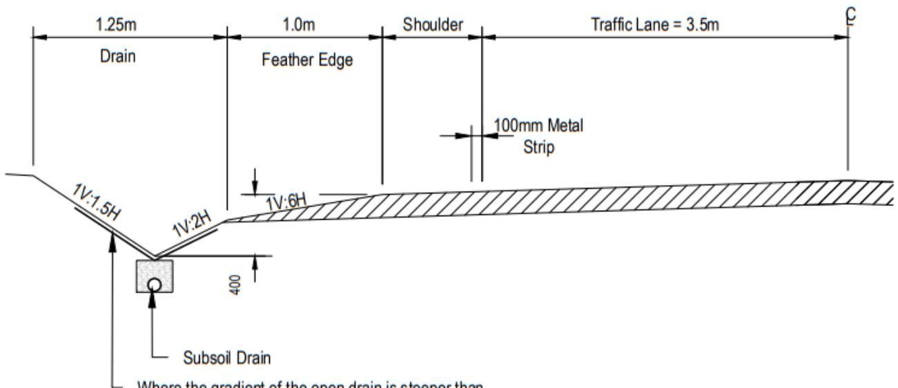
Where the gradient of the open drain is steeper than 1V in 15H or where soil type has the potential to erode use "Enkamat W" or similar
