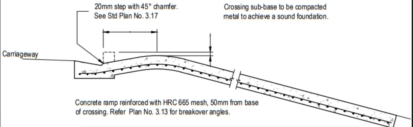
Concrete ramp reinforced with HRC 665 mesh, 50mm from base
