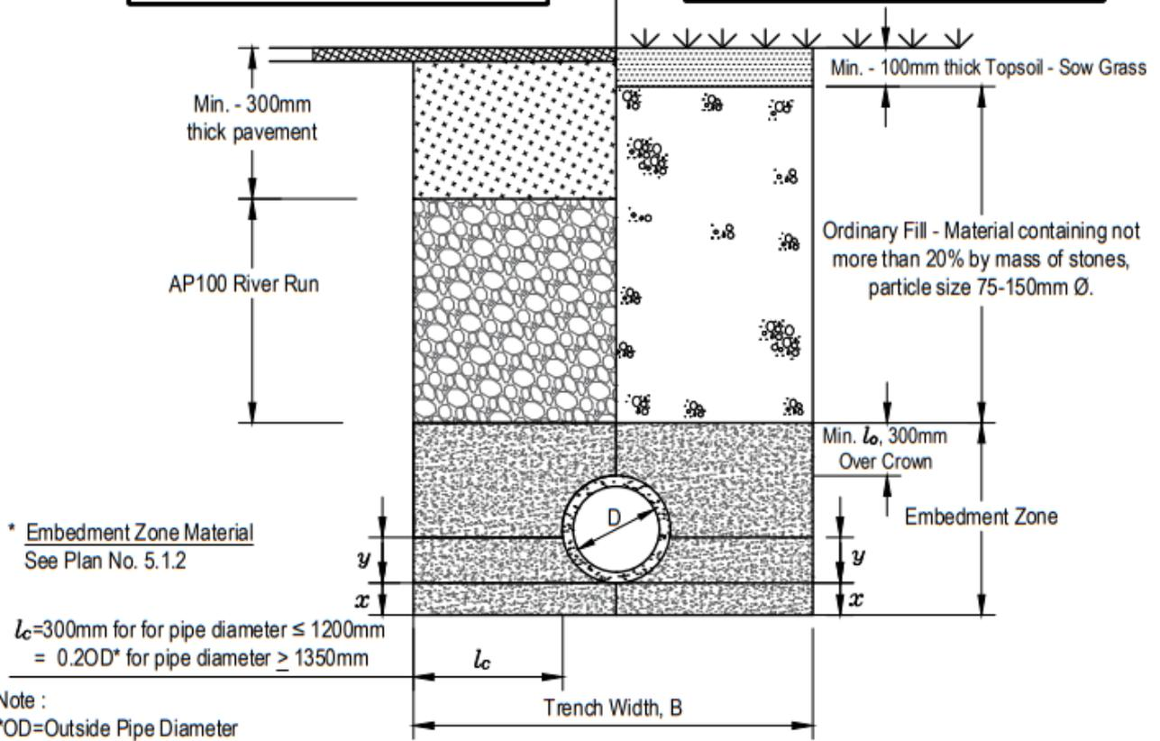
**CONCRETE OR CERAMIC PIPES**
