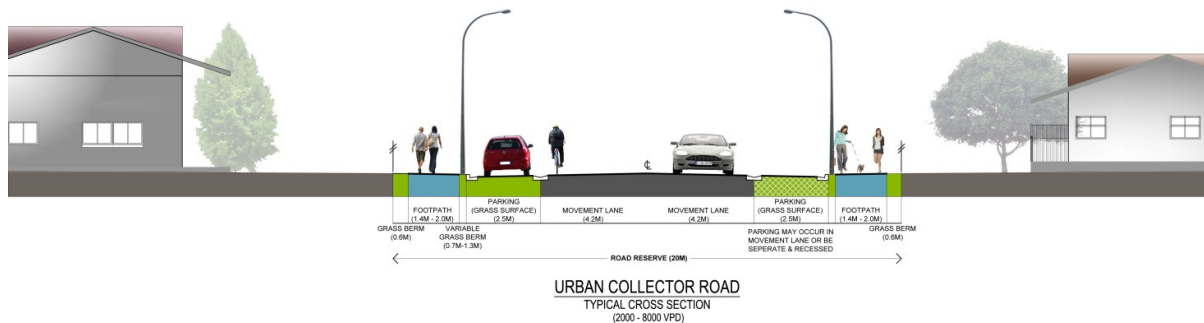
Figure 6-2: Urban Collector Road – Typical Cross-Section
