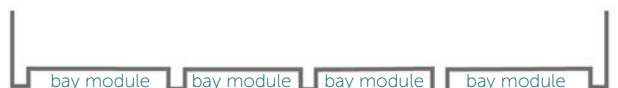
In plan view, modulation can be seen as a series of bay modules formed by projecting and recessive elements.
