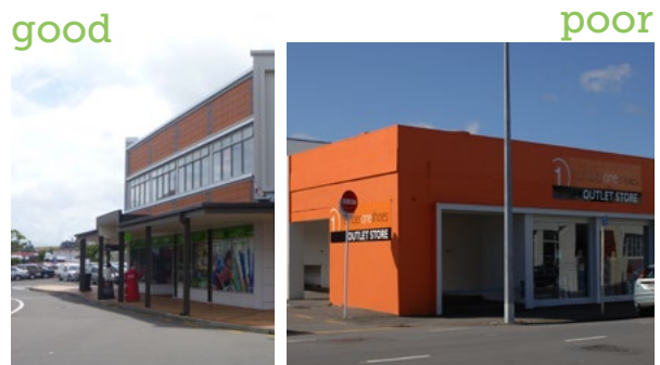
The verandahs of the BNZ building (left) are good as they extend the width of the footpath and are supported by posts. Although a modern interpretation, the BNZ example also shows a parapet line and extended vertical structural features at the corners. The building entrance is emphasised with a change in verandah height. The example on the right is poor as it has no verandah and has no parapet features.
