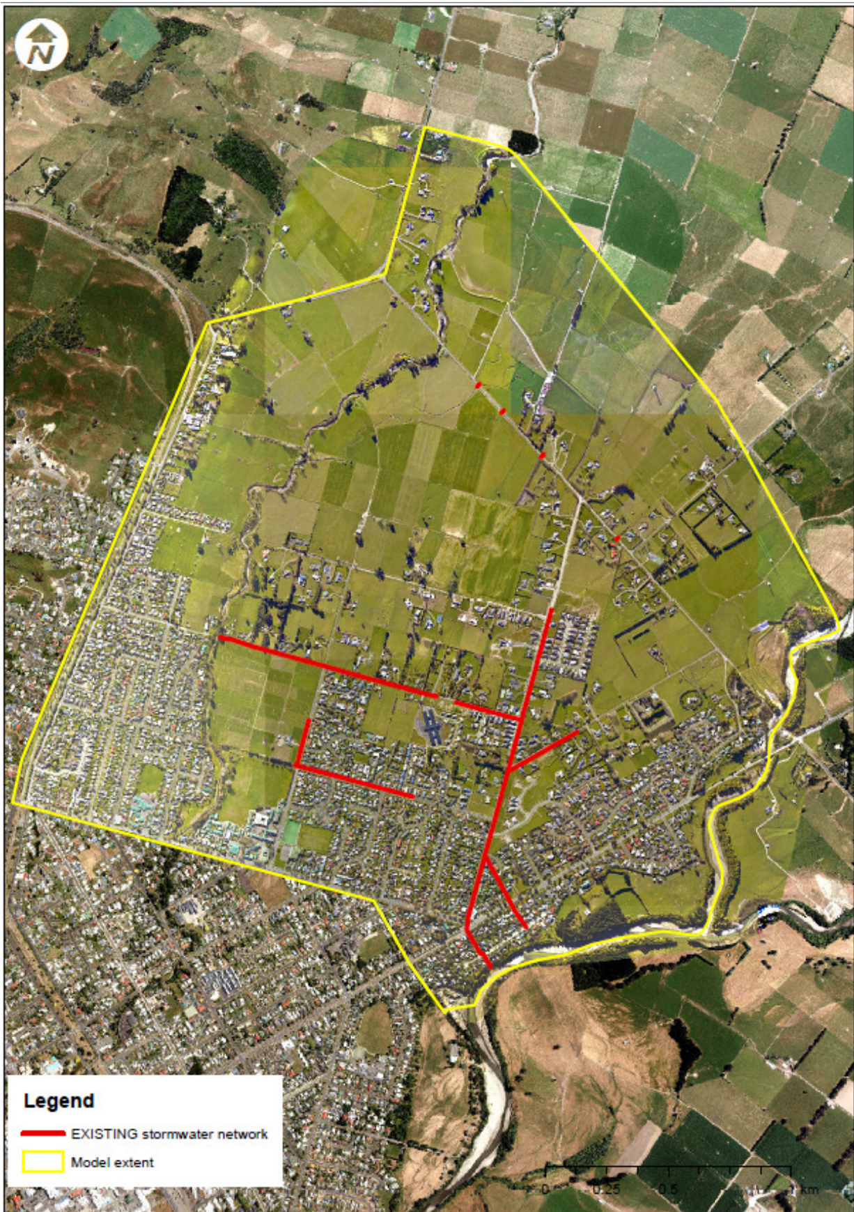
Figure B-1-0-1: Existing stormwater infrastructure within Precinct 4 included in the 2-D model
