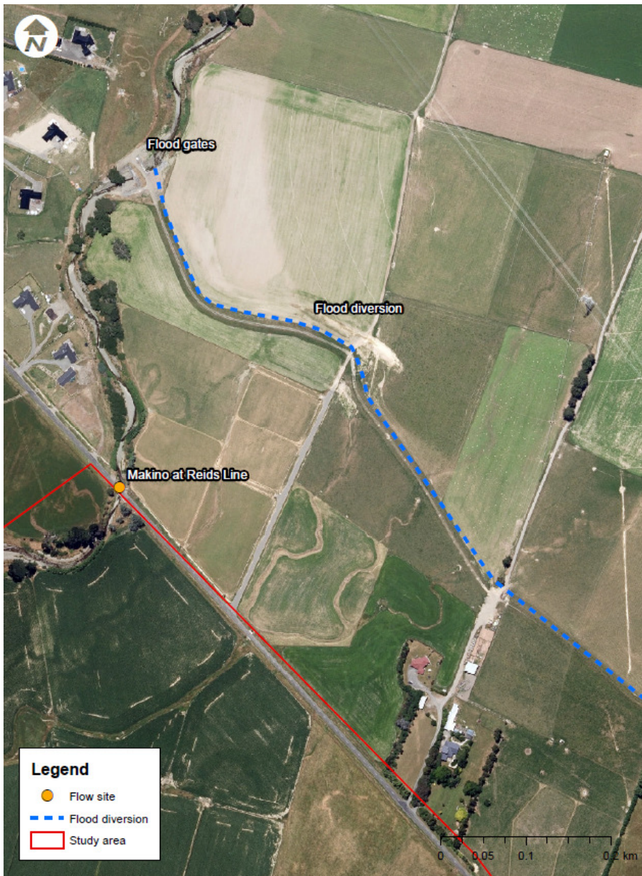
Figure C-1-6: The Makino River flood control gates, diversion and flow monitoring site at Reid’s Line.
