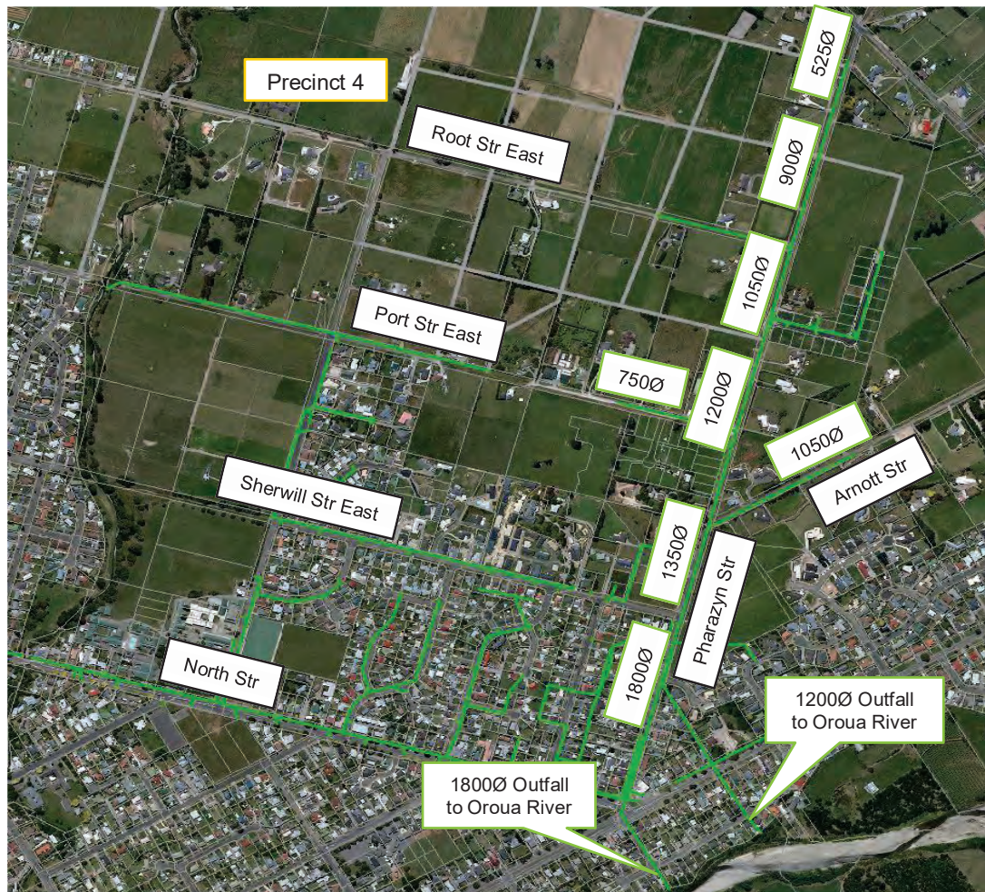
Figure 1 - Existing stormwater infrastructure
