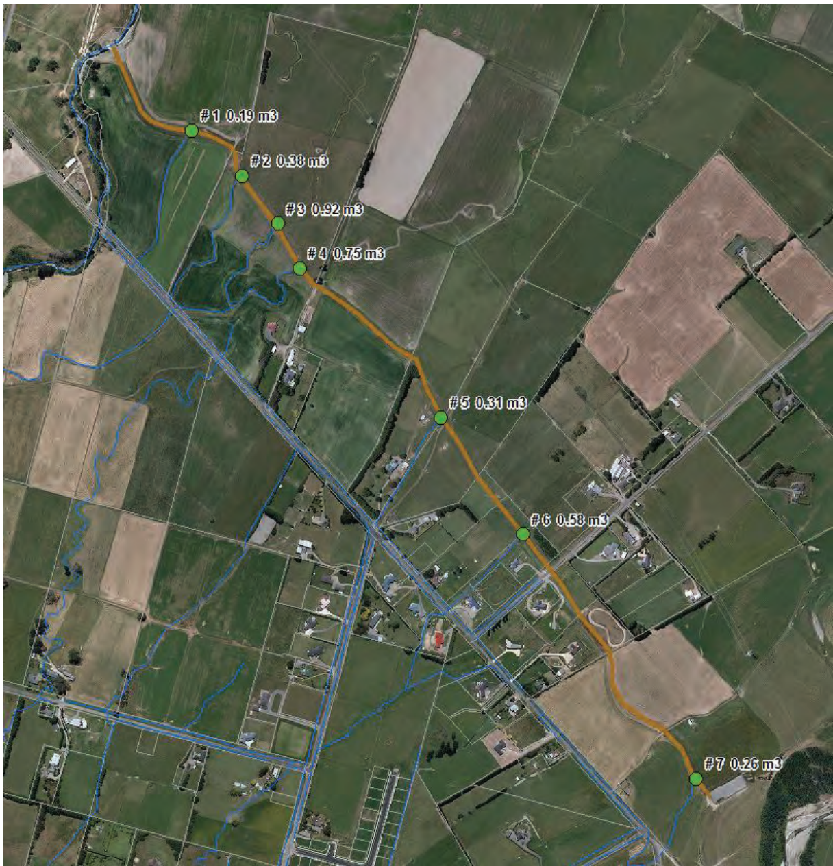
Figure 17 - 1 in 30-year stopbank flows entering Precinct 4
