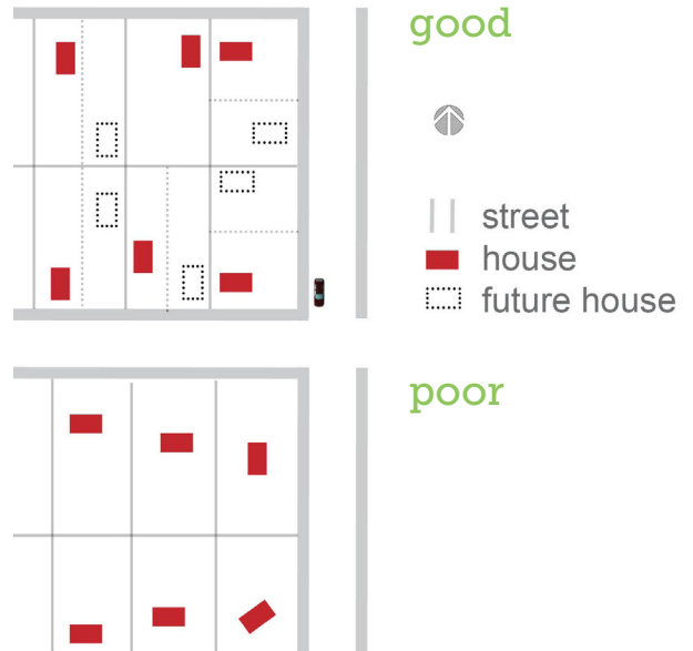
Diagram shows good arrangement of lots and house sites for the larger lot areas to enable later additional density. The poor example shows house sites not well located in terms of providing for future houses.
