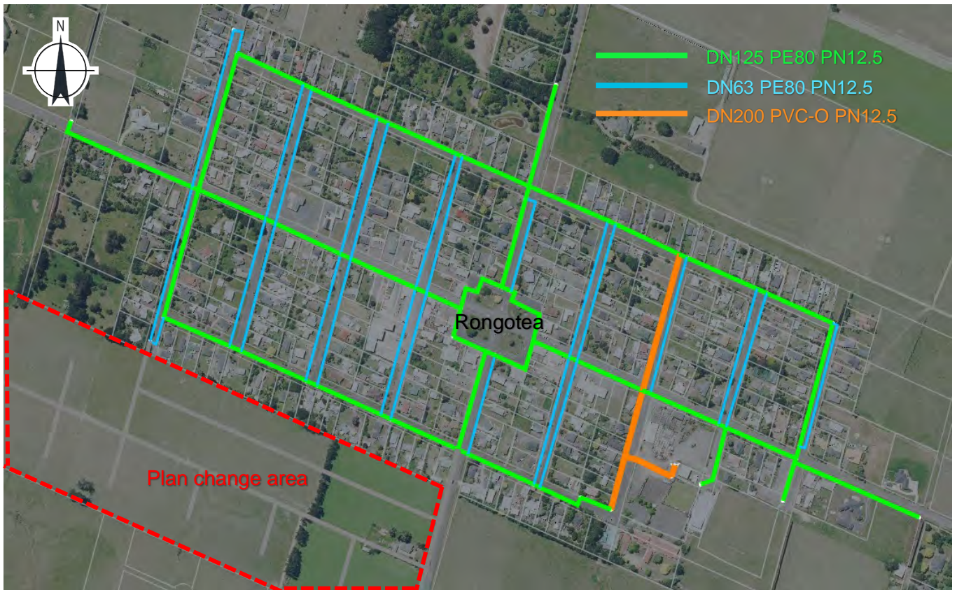
Figure 20 Rongotea existing water reticulation layout
