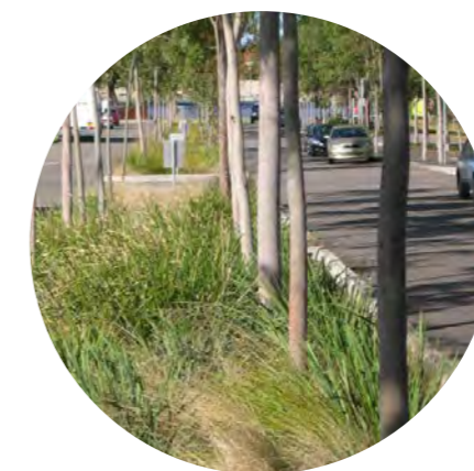
The use of landscaping in the streetscape supports stormwater retention and filtration to reduce flooding and improve water quality.
