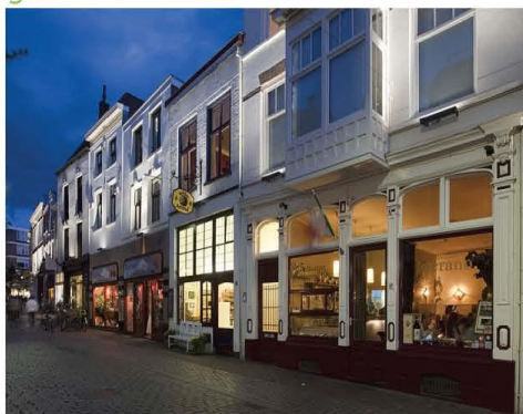
The example (above) shows lighting used on the facade to highlight the continuous building line, and depth of features such as windows and pediment lines. Internal lighting highlights the shop content and reflects light to the street.
