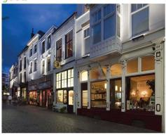
The example (above) shows lighting used on the facade to highlight the continuous building line, and depth of features such as windows and pediment lines Internal lighting highlights the shop content and reflects light to the street.
