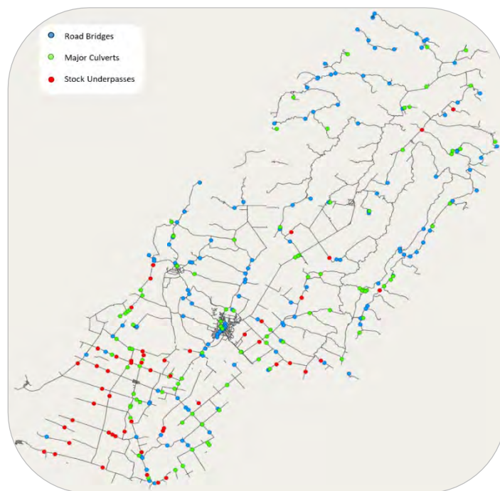
FIGURE 19: BRIDGE STRUCTURES ASSET MAP
