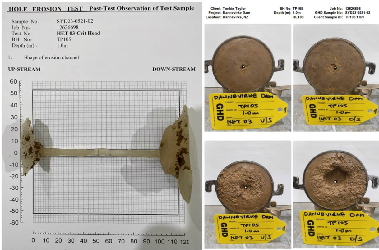
Figure 2-4: Example of post-test observations of a critical head HET on a remoulded sample from TP105 at 1.0m.
