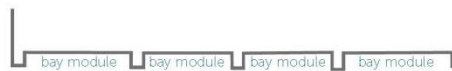
In plan view, modulation can be seen as a series of bay modules formed by projecting and recessive elements.
